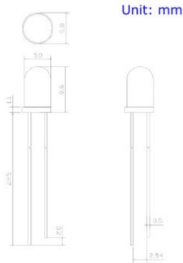
Finally, the mechanical drawing. This picture contains all of the measurements you'll need to actually mount the LED in an enclosure! Notice that, like most LEDs, this one has a small flange at the bottom. That comes in handy when you want to mount it in a panel. Simply drill a hole the perfect size for the body of the LED, and the flange will keep it from falling through!
