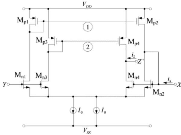
Fig.3 A differential pair based CMOS CCCII+ [10].
