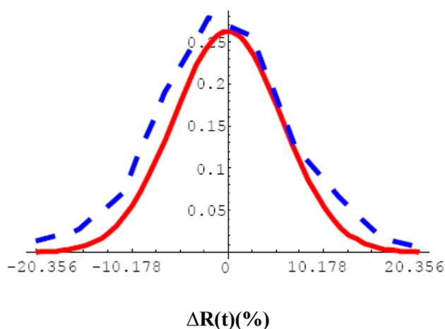
Fig.7: 90 nm based parameterized 1<sup>st</sup> order approximated  $\Delta R(t)$  distribution obtained from the proposed model (line) v.s. Monte-Carlo SPICE based counterpart obtained from the simulation of the candidate CMOS active resistor [11] at 90 nm level (dash)
