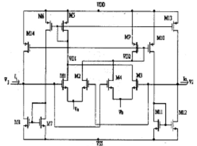
Fig.4 A CMOS active resistor proposed in [11].
