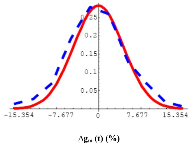
Fig.5: 90 nm based parameterized 1<sup>st</sup> order approximated  $\Delta g_m(t)$  distribution obtained from the proposed model (line) v.s. Monte-Carlo SPICE based counterpart obtained from the simulation of CMOS-OTA [9] at 90 nm level (dash)
