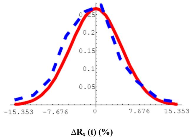
Fig.6: 90 nm based parameterized 1<sup>st</sup> order approximated  $\Delta R_x(t)$  distribution obtained from the proposed model (line) v.s. Monte-Carlo SPICE based counterpart obtained from the simulation of the candidate differential pair based CMOS CCCII+ [10] at 90 nm level (dash)
