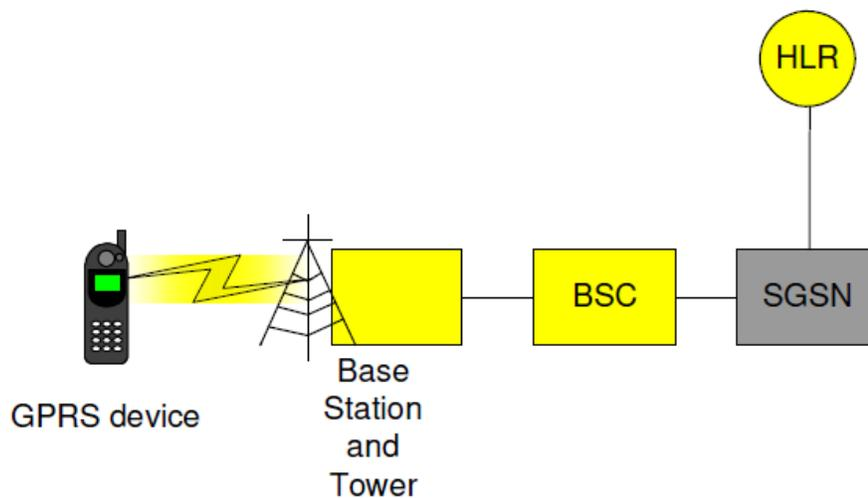
As mentioned earlier GPRS is not a completely separate network to GSM. Many of the devices such as the base transceiver stations and base transceiver station controllers are still used. Often devices need to be upgraded be it software, hardware or both. When deploying GPRS many of the software changes can be made remotely.
