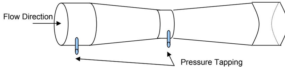
Figure 2: A Venturi Tube Flowmeter
