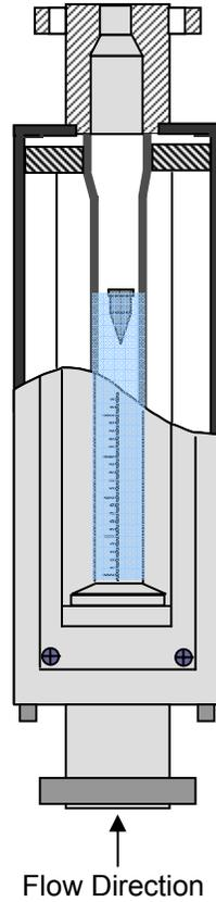
Figure 4: A Cross Sectional of Rotameter
