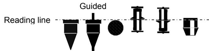
Figure 5: Typical Rotameter Bob Geometries
