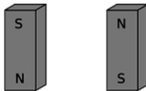
Figure e: Both magnets are reversed.
