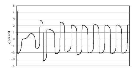
Figure 3.10 Example of ferroresonance voltages settling into a stable operating point (intersection 3) after an initial transient.
