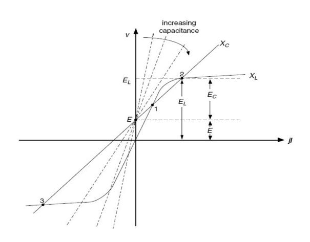
Figure 3.8 Graphical solution to the nonlinear LC circuit
