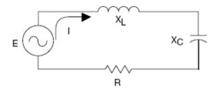
Figure 3.6 Simple series *RLC* circuit
