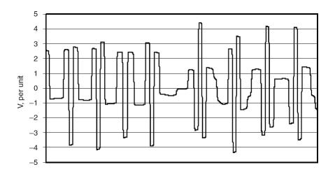
Figure 3.9 Example of unstable, chaotic ferroresonance voltages
