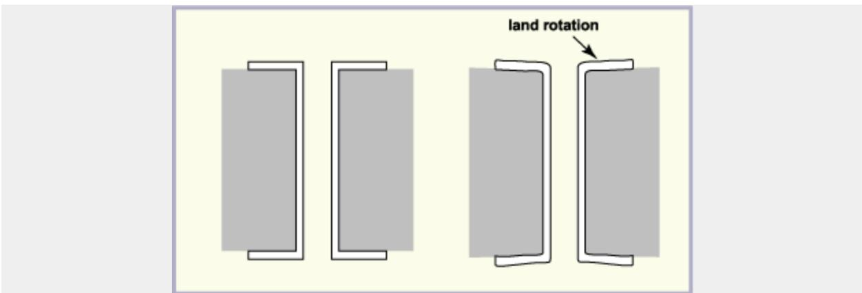
Because the stress exceeds the yield strength of copper, given sufficient temperature cycling, the cumulative strain will cause a crack in the copper barrel. This effect, referred to as 'ratcheting' is also seen in solder joints subjected to cyclical stresses.
