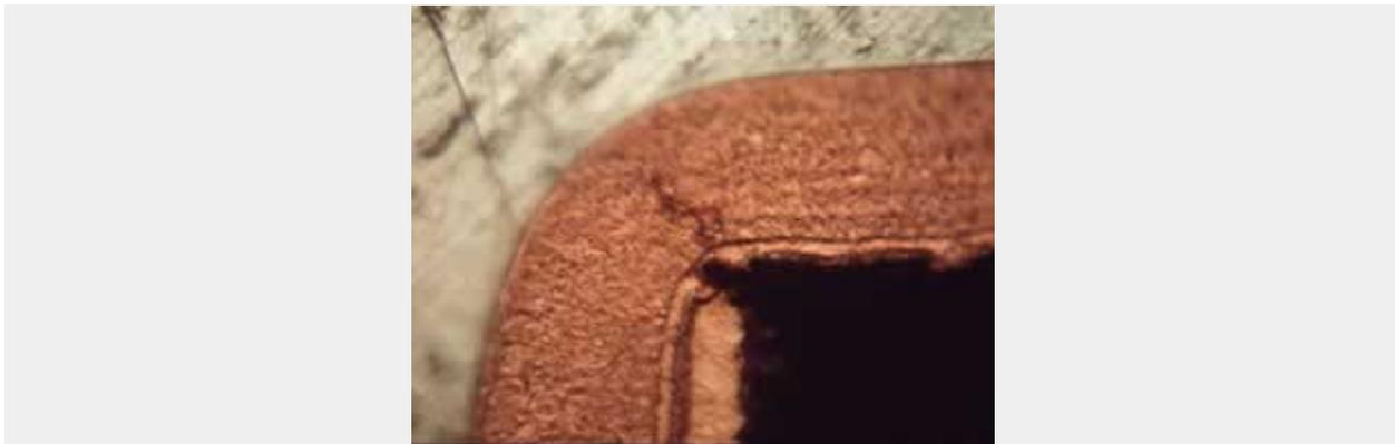
**Multi layer junction failure**
