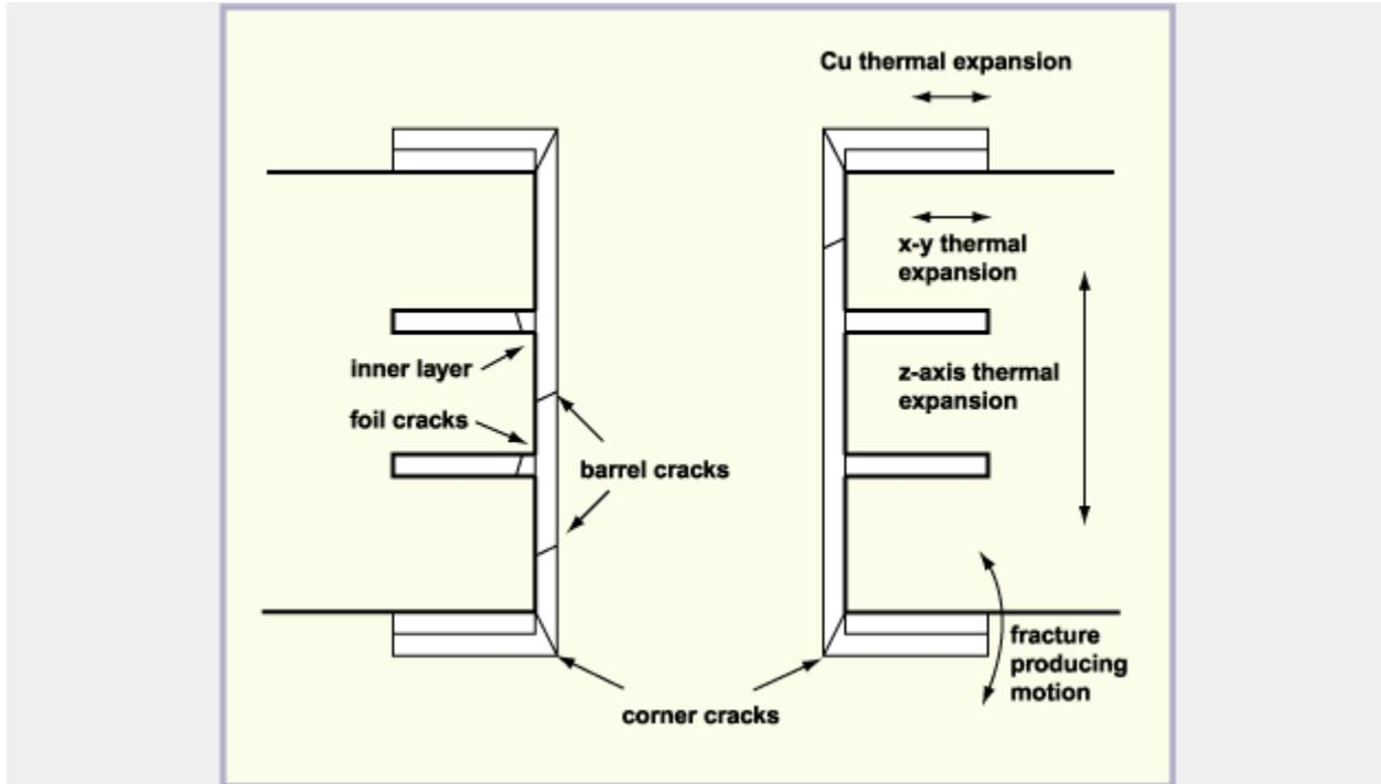
Illustrated in photographs are typical examples of corner cracking and inner layer cracks. Notice particularly that corner cracking starts from the stress point in the inside, rather than the outside, and can be relatively harmless in appearance. However, given that cracks tend to propagate, intermittencies and open-circuits can be created in a number of places within the through-hole structure.
