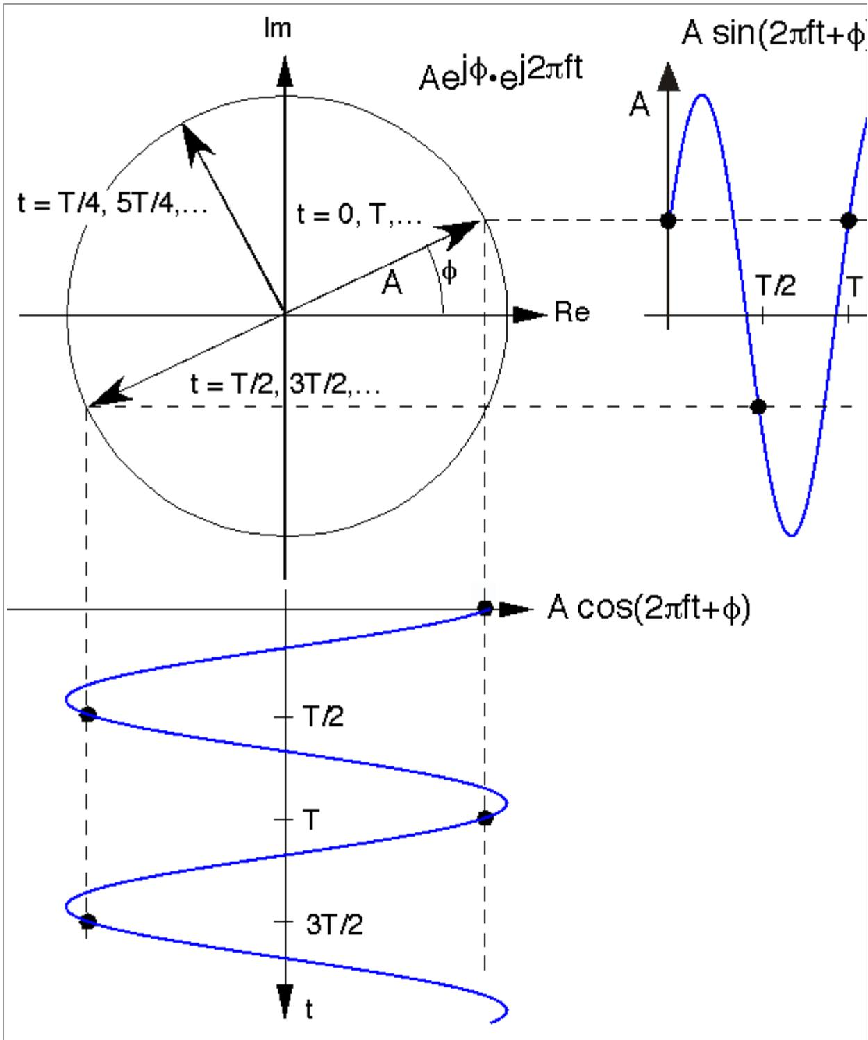
**Figure 1:** Graphically, the complex exponential scribes a circle in the complex plane as time evolves. Its real and imaginary parts are sinusoids. The rate at which the signal goes around the circle is the frequency  $f$  and the time taken to go around is the **period**  $T$ . A fundamental relationship is  $T=1/f$ .
