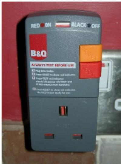
You can also buy plug-in RCD adapters. You plug these into the mains socket and then plug your mains powered equipment into the adapter, or you can get ones that replace the plug on your equipment. If you have your own lab / shed / home office that you use for your electrical work then it can be a good idea to use these on all the sockets in that room but at a minimum I'd recommend using one whenever you first connect your circuit to the mains or when performing any live testing.
