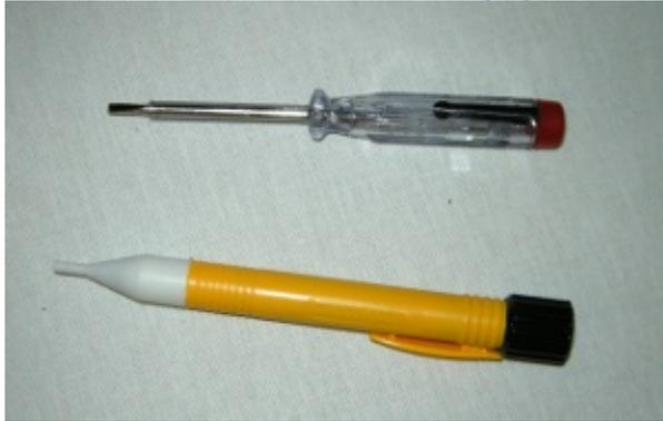
The most common type of **domestic** electrical tester is in the shape of a screwdriver with a neon inside the handle. You place the tip of the screwdriver on the contact you want to test and touch a metal plate at the other end of the screwdriver. If the tester is in contact with a mains voltage then the neon lights up. Always check that the tester is undamaged beforehand. Do not use these as a screwdriver.
