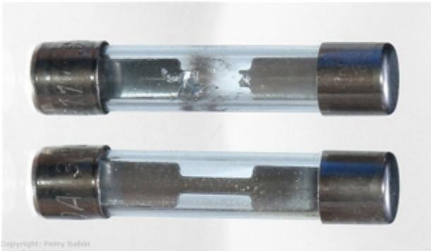
When there is an over surge that causes the fuse element to blow off, you can replace it. A new fuse carrier is inserted in the base.
