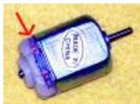
must be very careful if you try to do this because it is very easy to tear the solder tab off of the motor.
