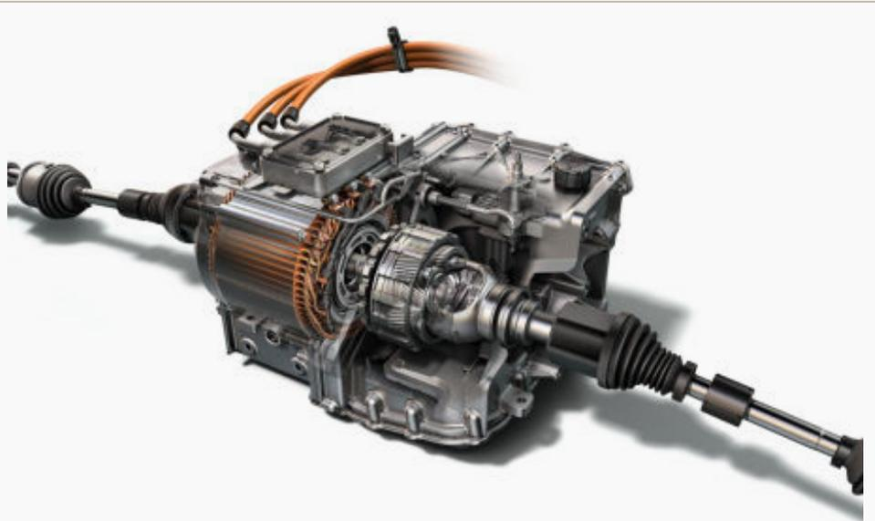
GM's new electric drive module in the 2014 Spark EV features a GM-designed-and-manufactured 120-kW permanent magnet traction motor (visible on the left side) and smart use of key carryover components from Volt and the two-mode hybrid transmission.
