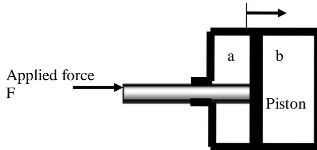
The basic operation of a dashpot, in which the housing is filled with oil. If a force  $f$  is applied to the shaft, the piston presses against oil increasing the pressure on side 'b' and decreasing pressure side 'a'. As a result the oil flows from side 'b' to side 'a' through the wall clearance. The friction coefficient  $B$  depends on the dimensions and the type of oil used.
