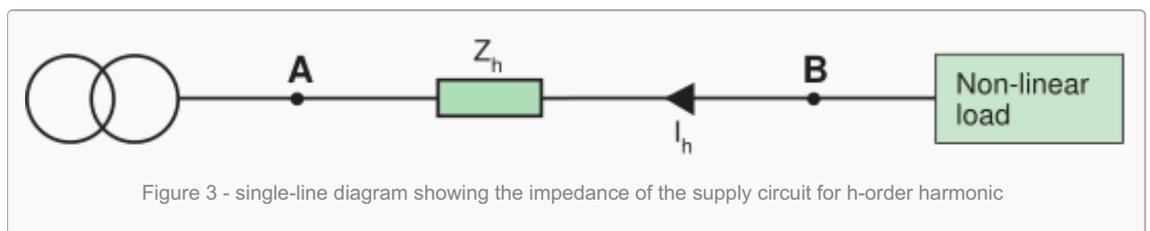
The h-order harmonic current creates via impedance  $Z_h$  a harmonic voltage  $U_h$ , where  $U_h = Z_h \times I_h$ , i.e. a simple application of Ohm's law. The voltage at **B** is therefore distorted and all devices supplied downstream of point **B** will receive a distorted voltage.
