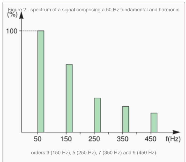
To better understand harmonic currents, it may be useful to imagine that the non-linear loads reinject harmonic currents upstream into the distribution system, in the direction of the source.
