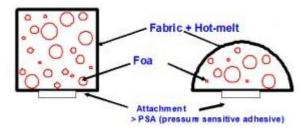
Figure 5. Fabric-over-foam (FoF) cross section.
