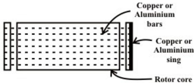
**Fig. 30.3(a): Squirrel cage rotor of induction motor**
