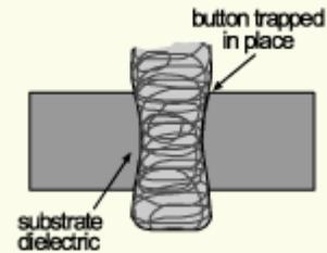
The contact has very low resistance and inductance, so is useable at microwave frequencies, and its very low mass and lack of resonance makes it resistant to shock and vibration.
