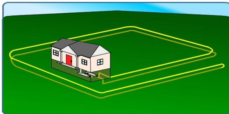
Horizontal Closed-Loop System - Two Pipe Layout
