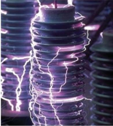
Arc quenching is also known as Arc Interruption or Arc Extinction theory. Let's talk about a few characteristics of the arc column in question. **Gas particles** are moving with speed and have a random motion at high temperature. Also in the absence of an electric field net motion is observed in the **gas particles**. Hence when the **gas particles** are provided with an electric field the particles gain a drift velocity in addition to their random movement.
