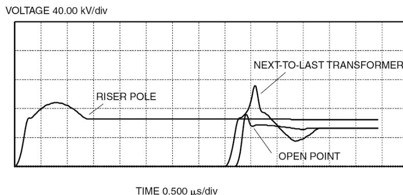
**Figure 4.36** Impulse voltages along a cable with an open-point arrester showing that the peak can occur at the next-to-last transformer. Simulation with UD Surge computer program
