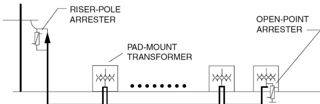
**Figure 3.28** Typical UD cable arrester application
