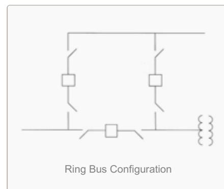
Arranging the scheme in this manner will minimize the potential for the loss of the supply to the ring bus due to a breaker failure. Relaying is more complex in this scheme than some previously identified. Since there is only one bus in this scheme, the area required to develop this scheme is less than some of the previously discussed schemes. However, expansion of a ring bus is limited, due to the practical arrangement of circuits.
