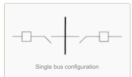
Maintenance of the bus would require the outage of the total system, use of standby generation, or switching to adjacent station, if available. Since the single bus arrangement is low in reliability, it is not recommended for heavily loaded substations or substations having a high availability requirement.
