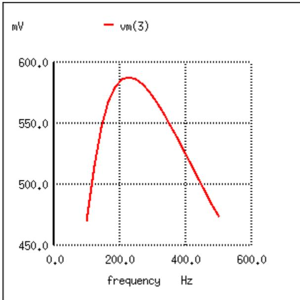
*The response of a capacitive bandpass filter peaks within a narrow frequency range. Band-pass filters can also be constructed using inductors, but as mentioned before, the reactive “purity” of capacitors gives them a design advantage. If we were to design a bandpass filter using inductors, it might look something like Figure [below](#).*
