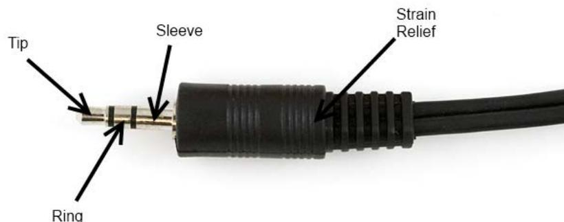
*Headphone-type TRS phone plug, 1/8". Typically, tip and ring will carry the stereo audio signals while sleeve will be connected to ground.*
