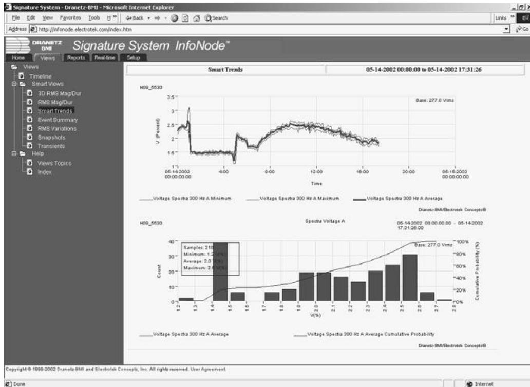
**Figure 5.13** On-line data analysis displayed on a standard Web browser. The analysis includes the trend of minimum, maximum, and average values of the fifth-harmonic voltage distortion along with a statistical distribution of the average values.
