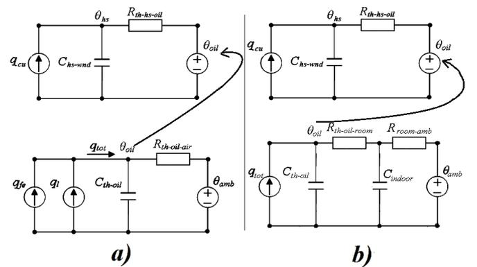
Fig. 6 Hot-spot temperature model a) Outdoor situation b) Indoor situation
