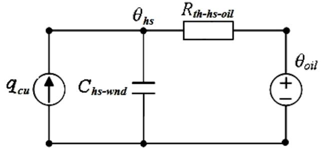
Fig. 5 Simplified Hot-spot temperature model
