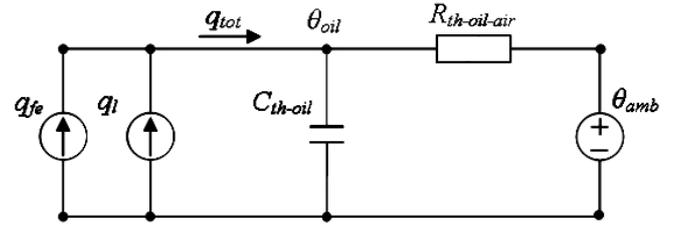
Fig. 2 The simplified equivalent top-oil thermal model
