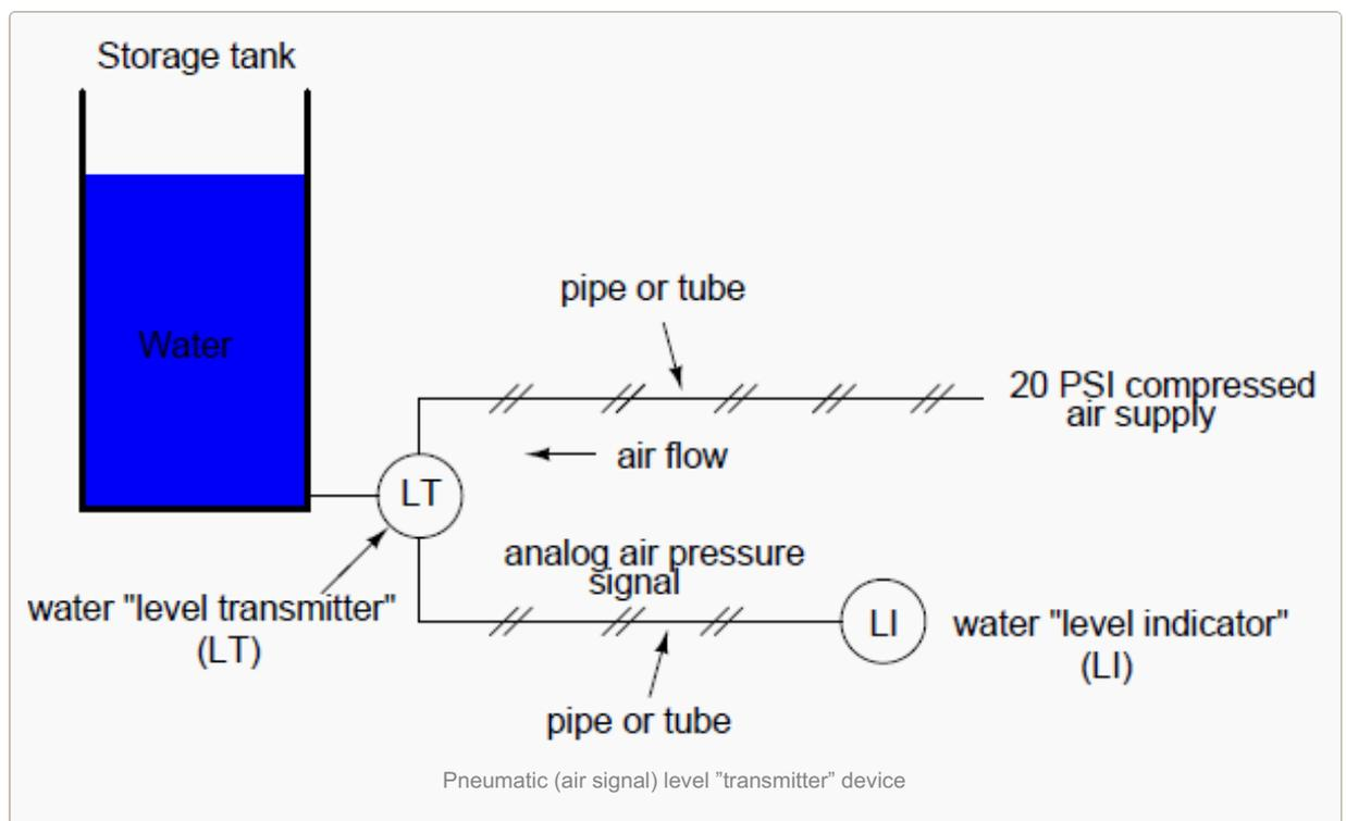
Air pressure signals are not only useful for measuring physical processes, but for controlling them as well. With a large enough piston or diaphragm, a small air pressure signal can be used to generate a large mechanical force, which can be used to move a valve or other controlling device.
