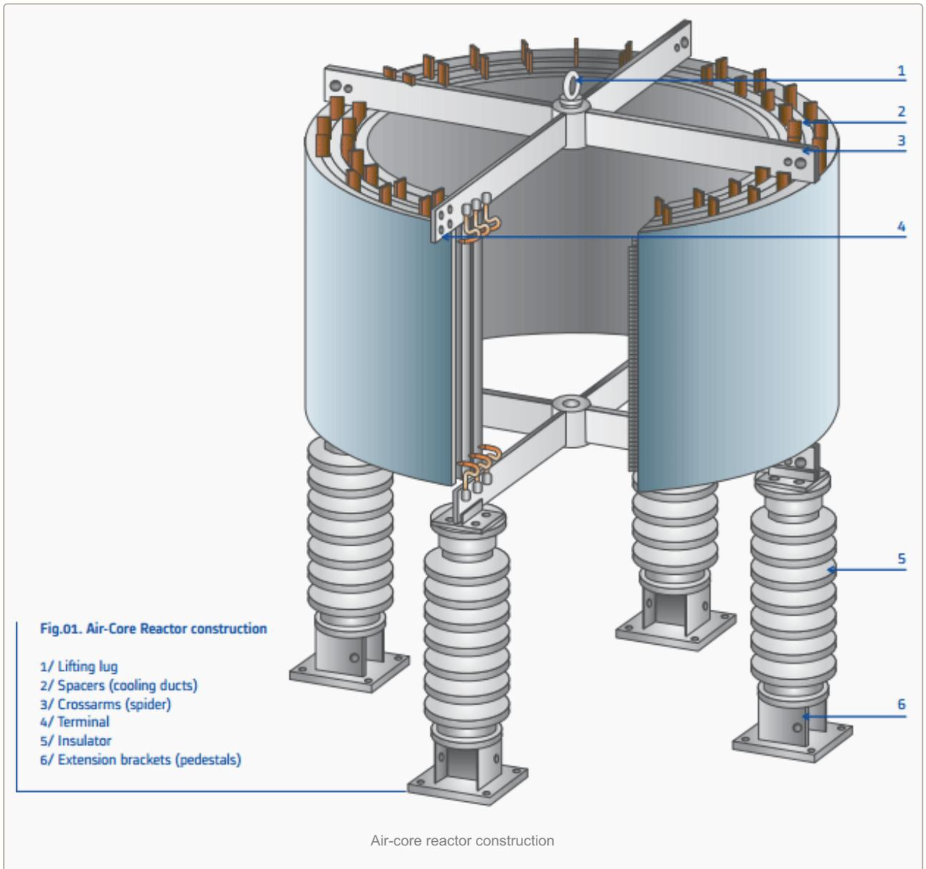
**reactors**, sound is generated by electromagnetic forces acting on the windings in a similar manner to that described above.
