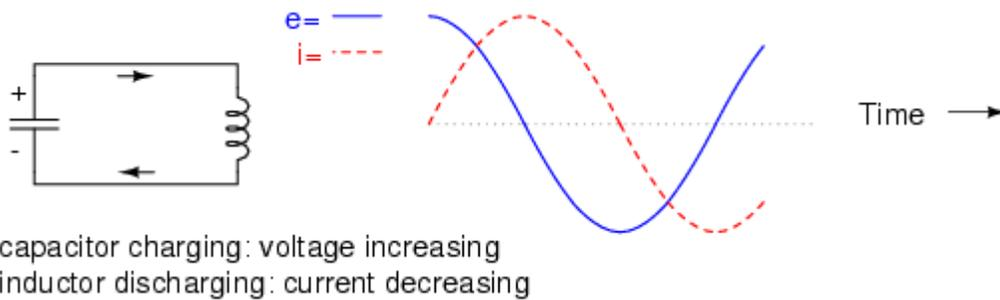
*Capacitor charging: voltage increasing, inductor discharging: current decreasing.* Eventually the capacitor will become fully charged again as the inductor expends all of its energy reserves trying to maintain current. The voltage will once again be at its positive peak and the current at zero. This completes one full cycle of the energy exchange between the capacitor and inductor: (Figure below)
