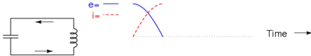
capacitor fully discharged: zero voltage
