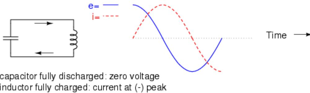
*Capacitor fully discharged: zero voltage, inductor fully charged: current at (-) peak.*
