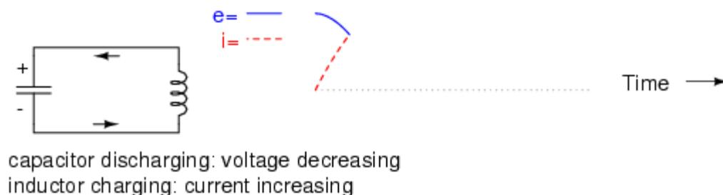
*Capacitor discharging: voltage decreasing, Inductor charging: current increasing.*
