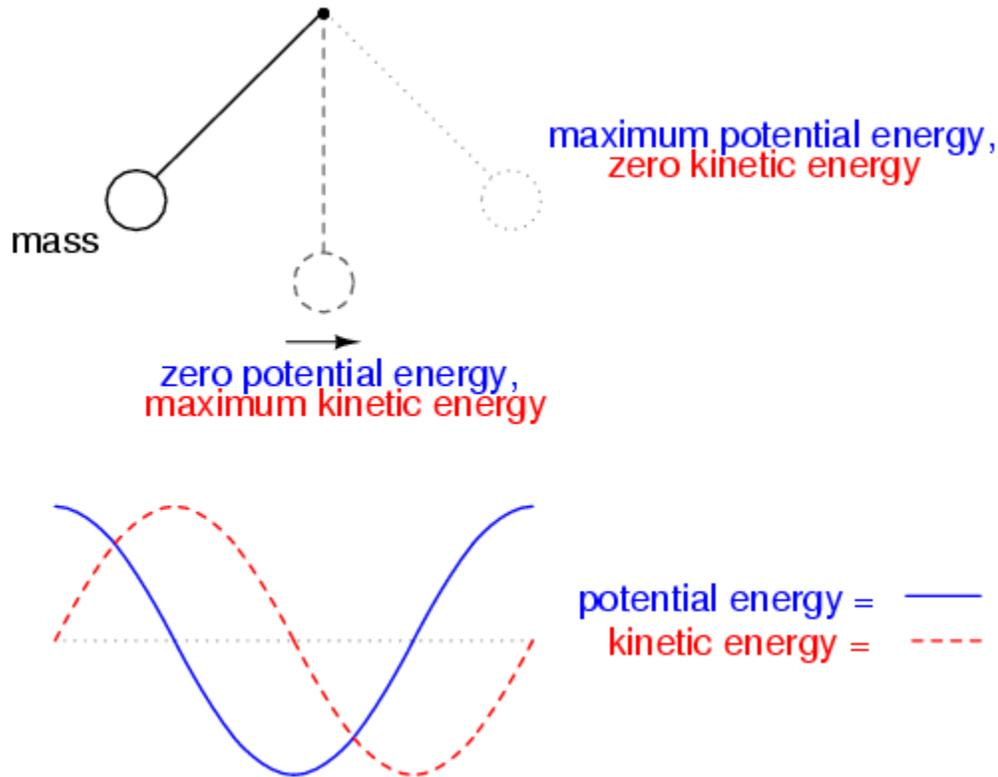
*Pendulum transfers energy between kinetic and potential energy as it swings low to high.*
