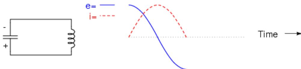
capacitor fully charged: voltage at (-) peak
