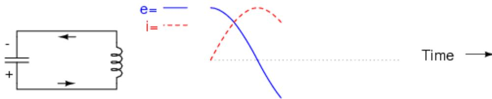
capacitor charging: voltage increasing (in opposite polarity)
