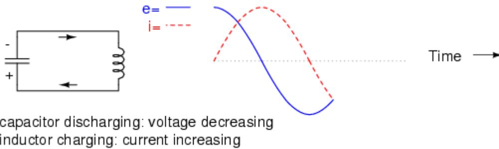
*Capacitor discharging: voltage decreasing, inductor charging: current increasing.*
