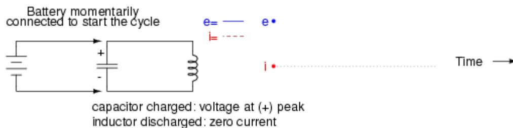
*Capacitor charged: voltage at (+) peak, inductor discharged: zero current.*
