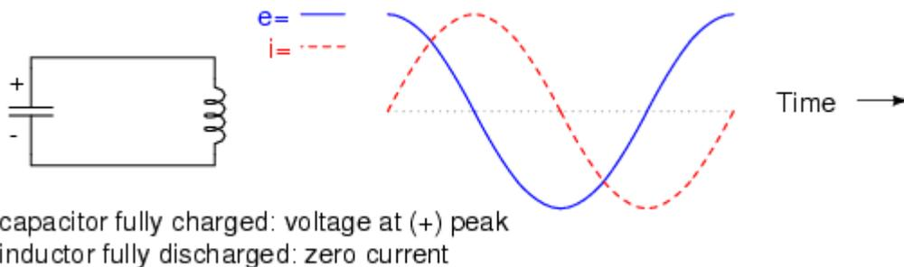
*Capacitor fully charged: voltage at (+) peak, inductor fully discharged: zero current.*
