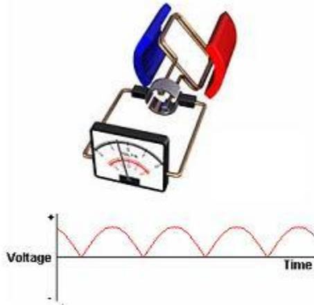
The above is a D.C. generator using a commutator. Notice that the voltage (e.m.f.) varies from zero to a maximum positive value.
