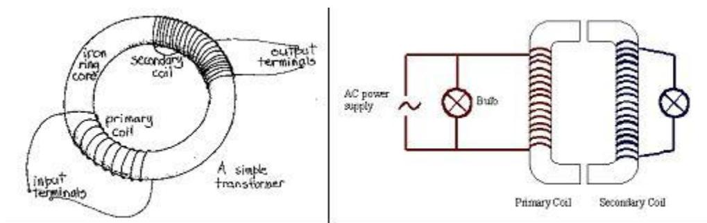
A transformer must still obey the law of energy conservation. In an ideal transformer the input power is equal to the output power. So if the transformer is used to step up the voltage the current must go down, if the transformer is used to step down the voltage the current must go up.
