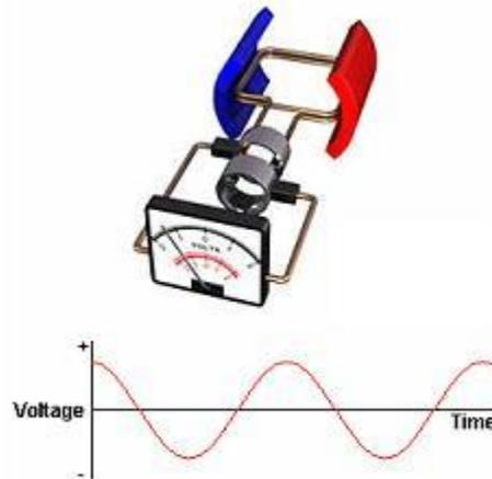
Above is an A.C. generator. No commutator is used, this causes the voltage (e.m.f.) to vary from a positive value to an equal but negative value.
