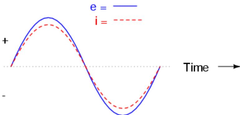
*Voltage and current "in phase" for resistive circuit.*
