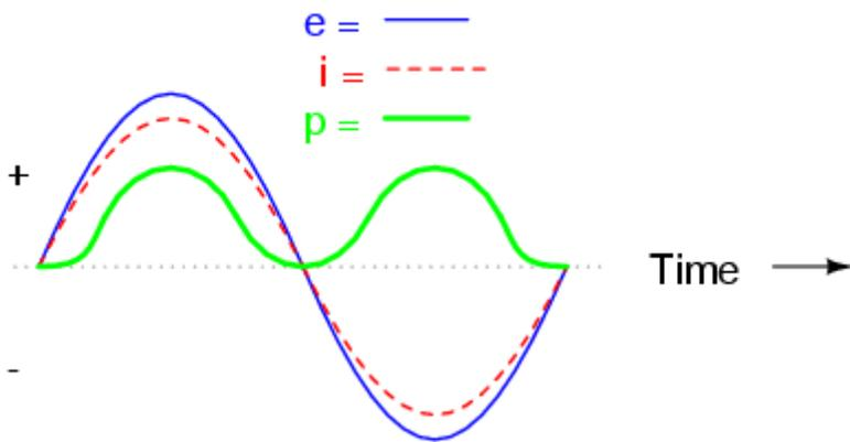
*Instantaneous AC power in a pure resistive circuit is always positive.*
