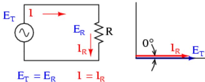
*Pure resistive AC circuit: resistor voltage and current are in phase.*
