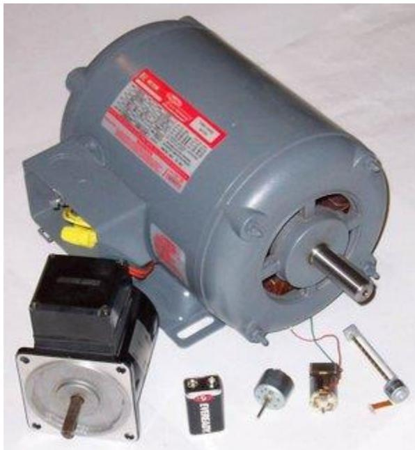
Three phase AC induction motors rated 1 Hp (750 W) and 25 W with small motors from CD player, toy and CD/DVD drive reader head traverse
