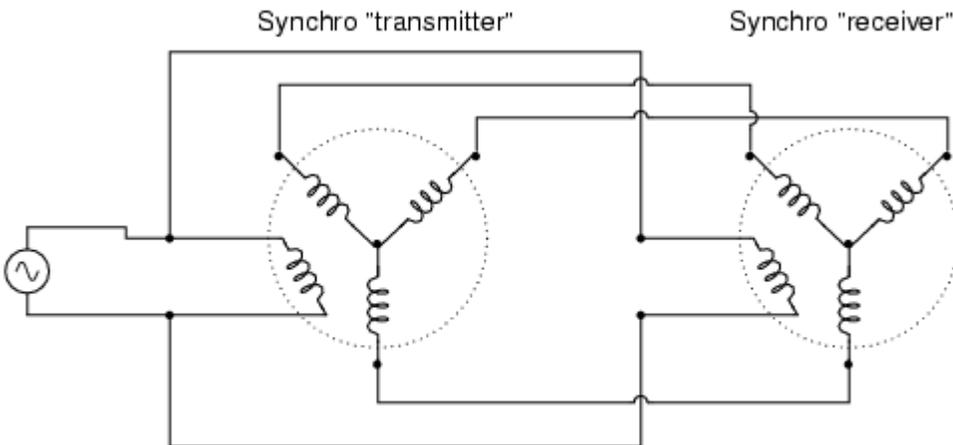
*The receiver rotor will turn to match position with the transmitter rotor so long as the two rotors remain energized.*
