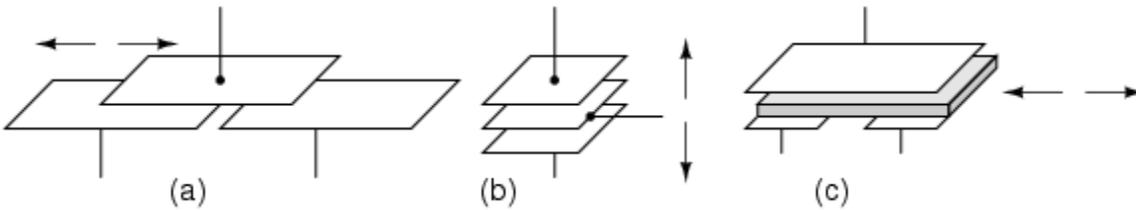
Differential capacitive transducer varies capacitance ratio by changing: (a) area of overlap, (b) distance between plates, (c) dielectric between plates.
