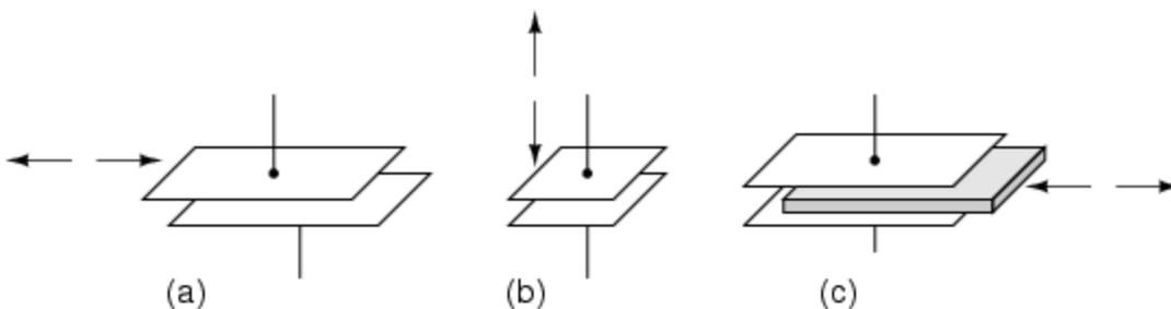
*Variable capacitive transducer varies; (a) area of overlap, (b) distance between plates, (c) amount of dielectric between plates.*
