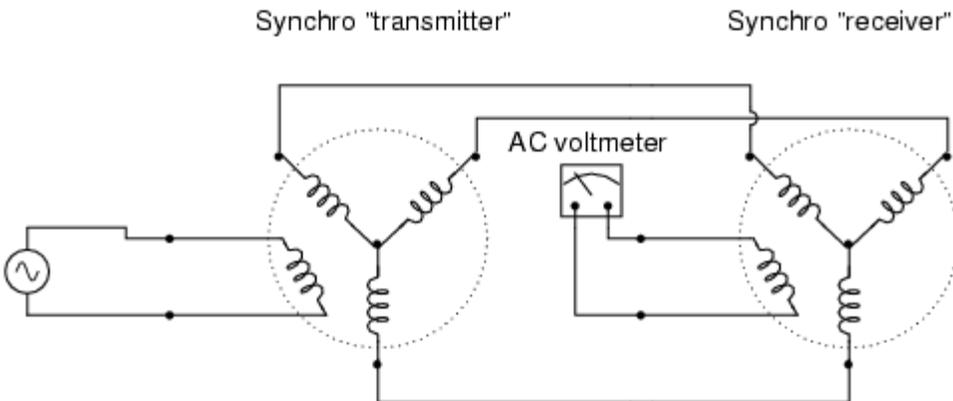
*AC voltmeter registers voltage if the receiver rotor is not rotated exactly 90 or 270 degrees from the transmitter rotor.*
