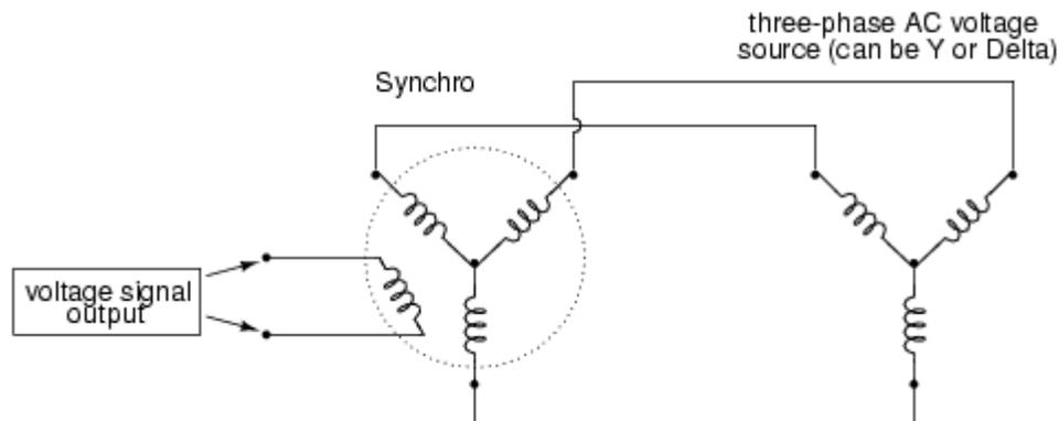
Full rotation of the rotor will smoothly shift the phase from  $0^\circ$  all the way to  $360^\circ$  (back to  $0^\circ$ ).
