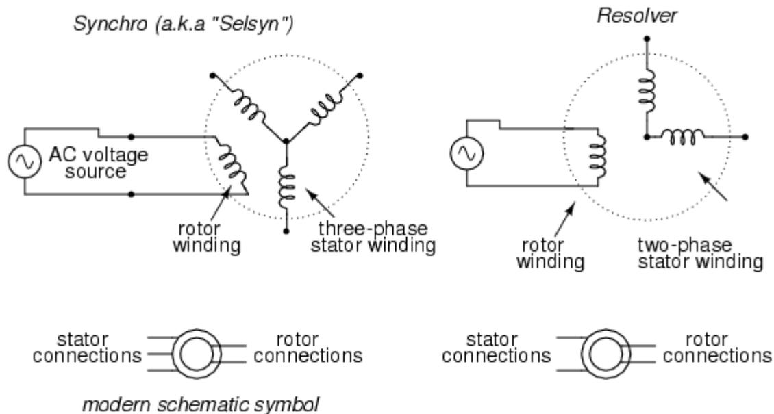
*A synchro is wound with a three-phase stator winding, and a rotating field. A resolver has a two-phase stator.*
