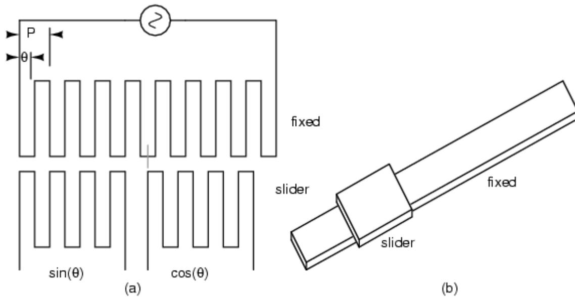
*Inductosyn: (a) Fixed serpentine winding, (b) movable slider 2-phase windings. Adapted from Figure 6.16 [WAK]*
