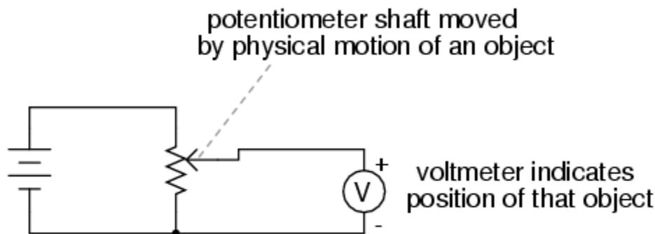
*Potentiometer tap voltage indicates position of an object slaved to the shaft.*
