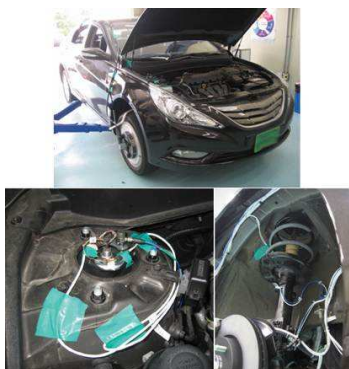
Fig. 3 Installation of the strain gauge-attached strut module on the car
