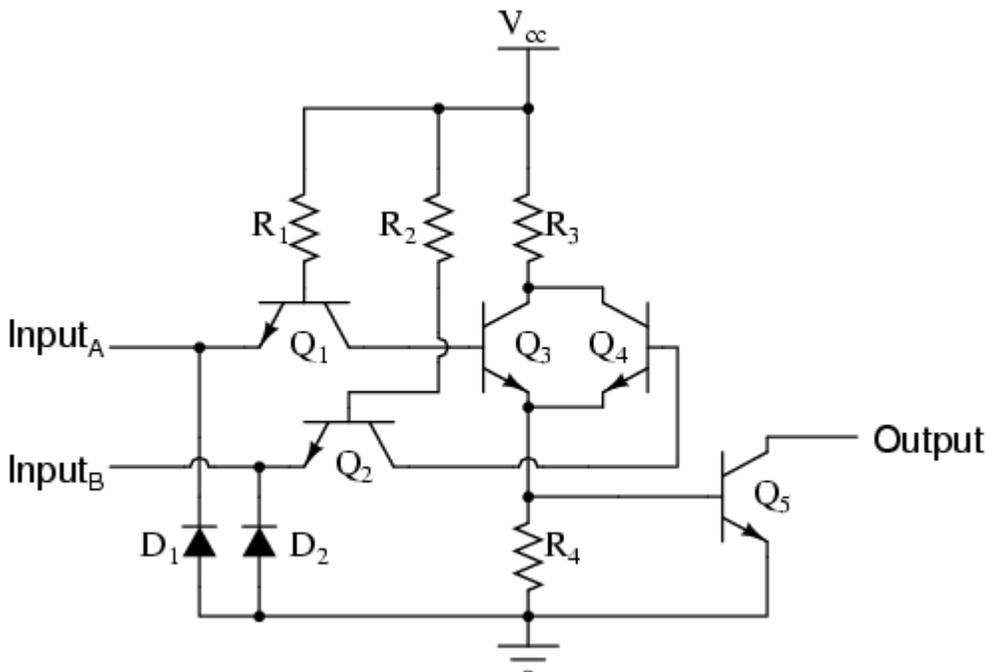
Transistors  $Q_1$  and  $Q_2$  are both arranged in the same manner that we've seen for transistor  $Q_1$  in all the other TTL circuits. Rather than functioning as amplifiers,  $Q_1$  and  $Q_2$  are both being used as two-diode "steering" networks. We may replace  $Q_1$  and  $Q_2$  with diode sets to help illustrate:
