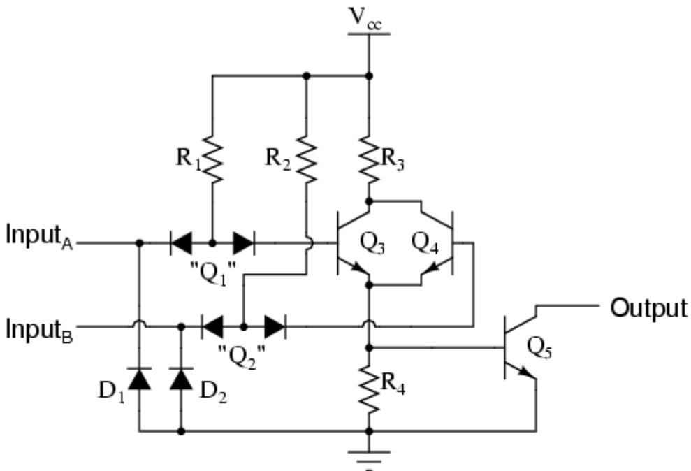
If input A is left floating (or connected to  $V_{cc}$ ), current will go through the base of transistor  $Q_3$ , saturating it. If input A is grounded, that current is diverted away from  $Q_3$ 's base through the left steering diode of " $Q_1$ ," thus forcing  $Q_3$  into cutoff. The same can be said for input B and transistor  $Q_4$ : the logic level of input B determines  $Q_4$ 's conduction: either saturated or cutoff.
