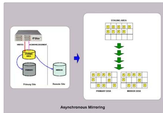
FIGURE 4: Asynchronous Mirroring
