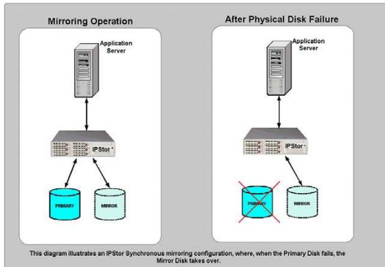
FIGURE 3: Synchronous Mirroring
