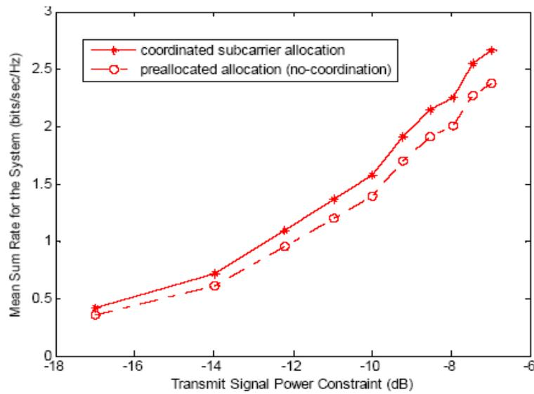
Figure 7: Comparison of two schemes for varying transmit power constraint (20mW to 200mW),  $ISD=500$ .
