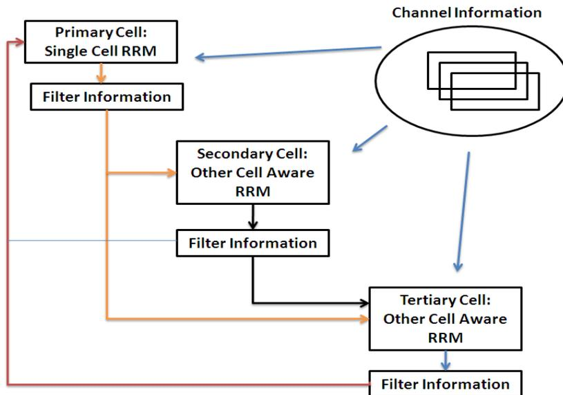
Figure 2: The sequence of resource allocation and information flow for the coordination scheme.
