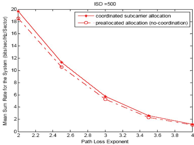
Figure 6. Comparison of the two schemes for various path loss environments.
