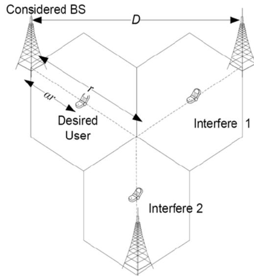
Figure 1: Illustrating reuse of resources if the three users are closer to their serving base station.
