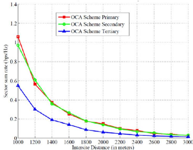
Figure 8: Comparison of the rate share for primary, secondary and tertiary sector in sequential Other Cell Aware Sub-band and Power Allocation
