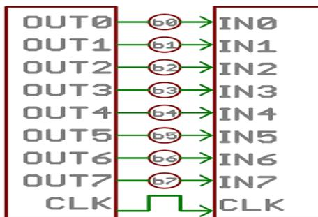
*An 8-bit data bus, controlled by a clock, transmitting a byte every clock pulse. 9 wires are used.*
