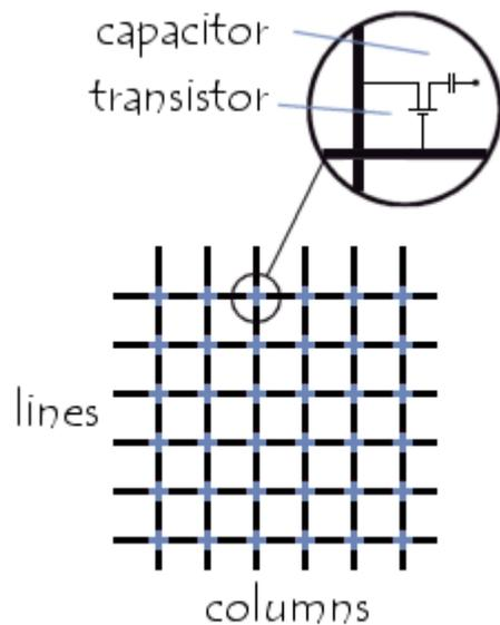
Each memory point is thus characterised by an address which corresponds to a row number and a column number. This access is not instant and the access time period is known as **latency time**. Consequently, time required for access to data in the memory is equal to cycle time plus latency time.
