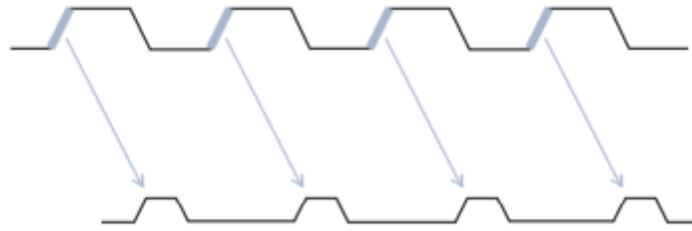
The DDR doubles the frequency of reading/writing, with a clock at the same frequency, by sending data to each leading edge and to each trailing edge.
