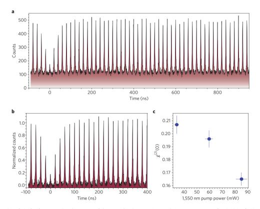
**Figure 4 | Upconversion of single photons. a**, Raw histogram of the second-order intensity correlation measurement after 3,600 s. **b**, Normalized second-order intensity correlation  $g^{(2)}(\tau)$  after ASR photon event subtraction. **c**,  $g^{(2)}(0)$  values with errors (see Methods) for different powers of the 1,550-nm pump laser.
