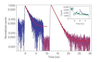
**Figure 3 | Time-resolved photoluminescence of a single quantum dot.** PL lifetime measured by the InGaAs SPAD (blue) and the silicon SPAD (maroon) after upconversion. Inset: raw histograms of the signal (blue) and dark count only (green) traces taken with the InGaAs SPAD.
