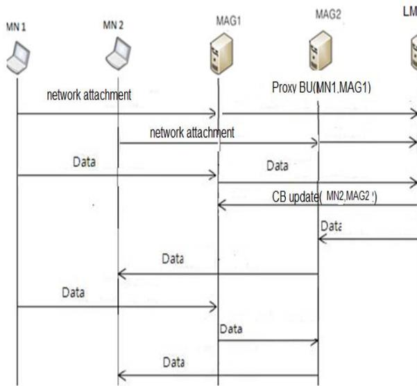
Fig1. Data flow in Light Weight RO Scheme
