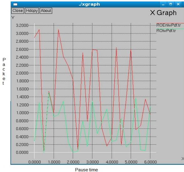
Fig 5 Packet delivery fraction comparison study graph
