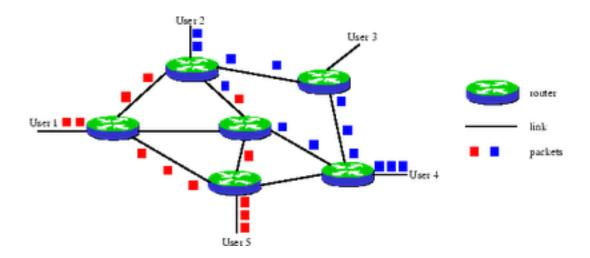
In datagram approach each packet is treated independently with no reference to packets that have gone before. So the packets each with same destination address do not follow the same route and they may arrive out of sequence at exit point. Hence exit node restores their packets to their original order before delivering them to destination.
