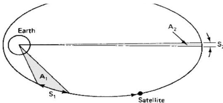
Figure 2.2 Kepler's second law. The areas  $A_1$  and  $A_2$  swept out in unit time are equal.
