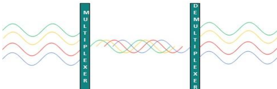
[Image: Wavelength Division Multiplexing]
