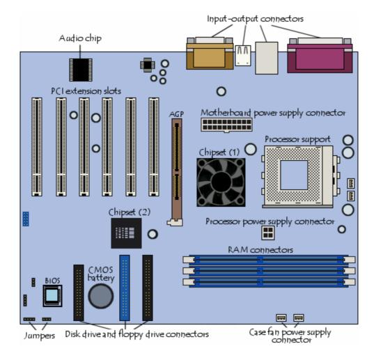
As its name suggests, the motherboard acts as a "parent" board, which takes the form of a large printed circuit with connectors for expansion cards, memory modules, the processor, etc.
