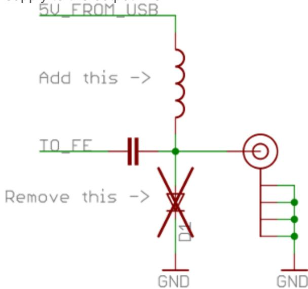
The modification allows to operate an active antenna without external components, but be sure not to connect any passive antenna shorted to ground, as that would quickly destroy the biasing inductor in the radio since there is no current limitation circuit (that's why my board looks so bad around the missing protection diode :-).
