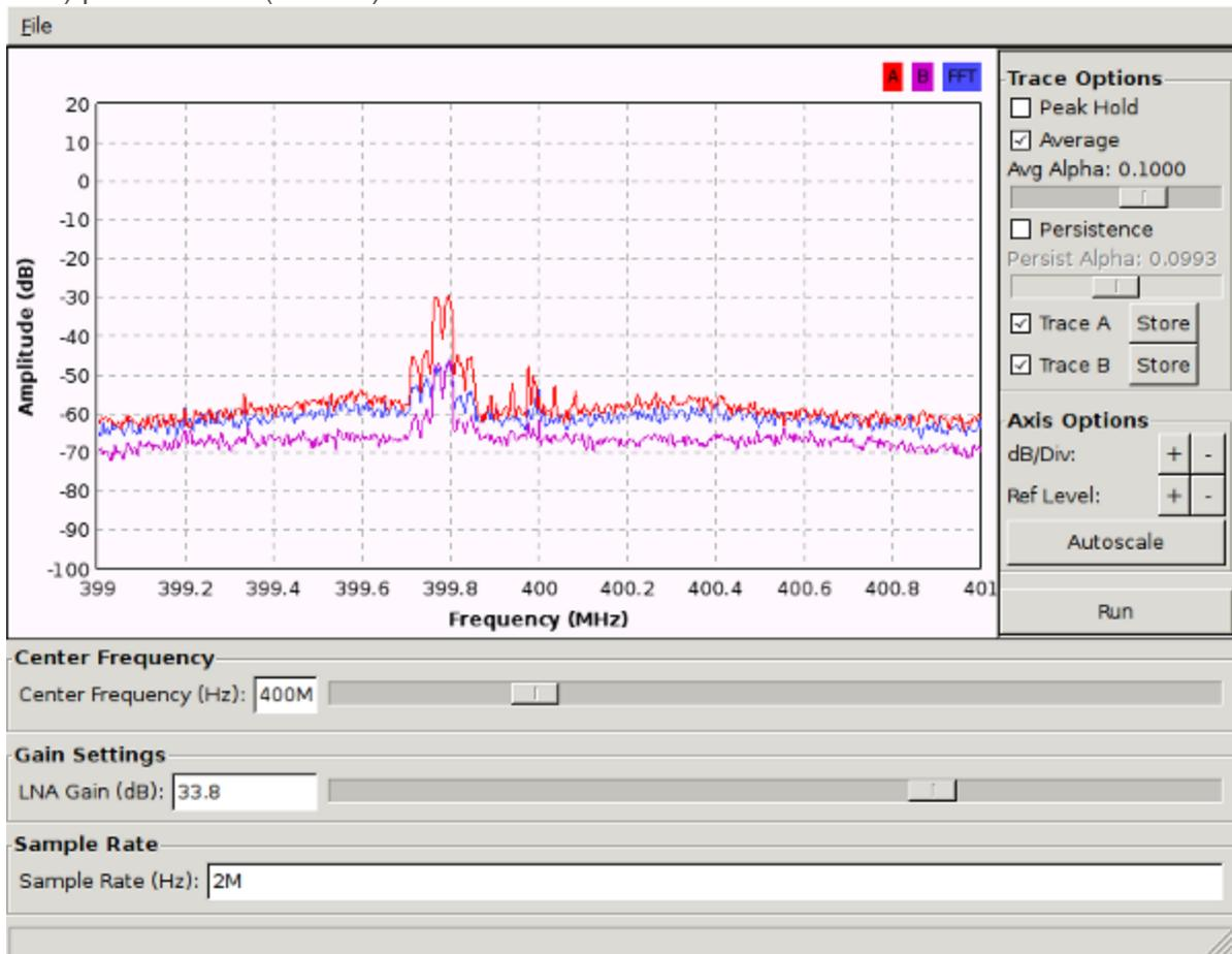
The results are quite good and show that the LNA is powerful enough to compensate for the loss for a cable of that length (about 20dB at 400MHz).
