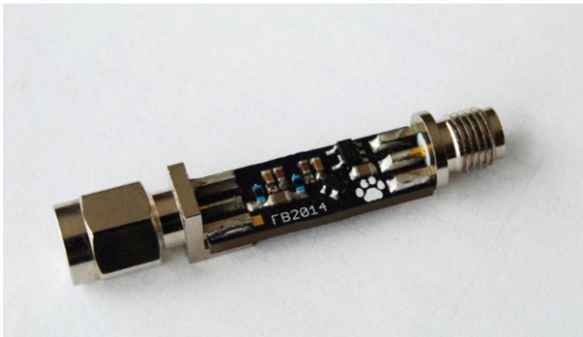
The LNA is based on the Mini Circuits PSA4-5043+, and the board is designed to be as small as possible to fit in line with the antenna and cable, and to be powered by the receiver itself.
