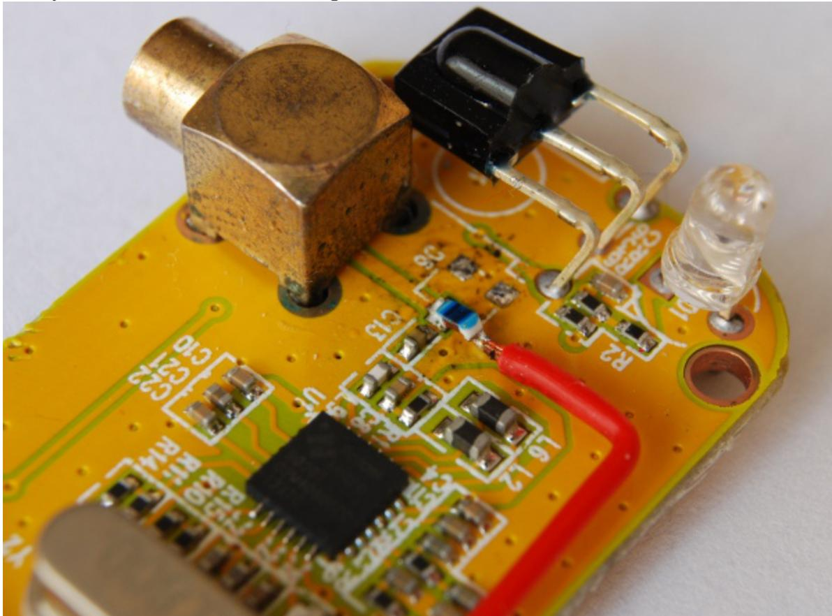
The modification involves first verifying the existing circuit to ensure that the input is already DC filtered (the series capacitor C13), then removing any existing clamping protection that would short the DC to ground (D8 in the picture) and finally mounting an inductor from the USB 5V supply to the output line.
