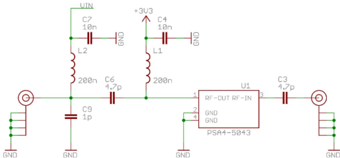
The two signal inductors are used to filter the DC power from the cable (L2), feed it to the linear regulator (not shown here) and feed a regulated DC (L1) back into the amplifier (U1). Optionally a third inductor may be connected from VIN to the antenna connector (after C3) to feed a DC supply back on the input cable, allowing for connection of multiple amplifiers in series.
