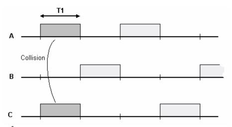
The mobile communication the user requests for a slot, using random access technique (ALOHA).
