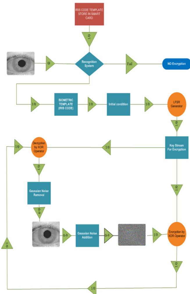
Figure 1. Proposed BGS cipher model.
