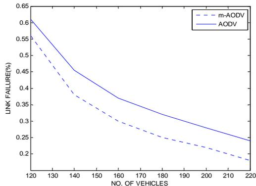
Fig 4 - Effect of no. of vehicles on link failure (%)
