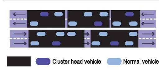
**FIGURE 1** Vehicles form multiple clusters in cluster-based routing.
