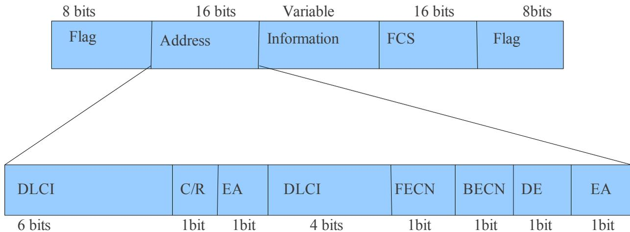
Fig:Frame Relay Frame Format
