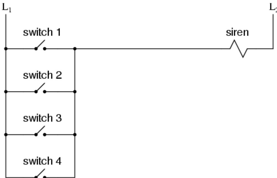
Essentially, this is the OR logic function implemented with four switch inputs. We could expand this circuit to include any number of switch inputs, each new switch being added to the parallel network, but I'll limit it to four in this example to keep
